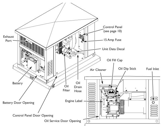
**I5 Amp Fuse** — Protects the DC control circuits.
